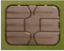
Figure 17.2: Smartcard integrated circuit chip shown from smartcard-enabled credit card
