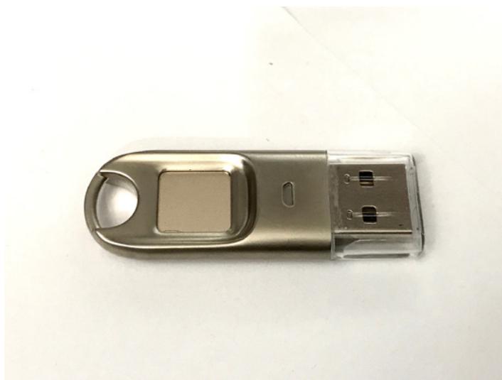
Figure 16.1: Fingerprint reader sensor incorporated on a relatively inexpensive FIDO (Fast ID Online) USB device
