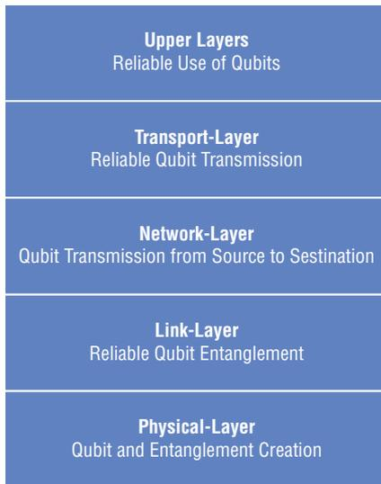
**Figure 8.4:** Proposed lower layers quantum network stack representation
