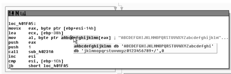
Figure 12-3: Following the cross-reference to the alphabet leads you to the base64 algorithm.
