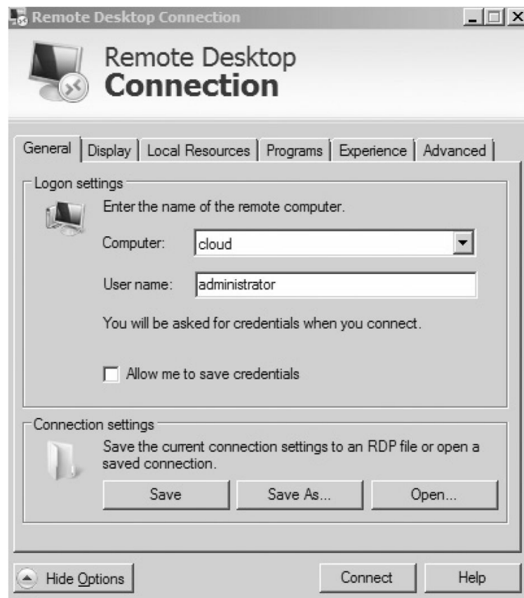
FIGURE 7-2 Remote Desktop Connection: An example of RDP software
