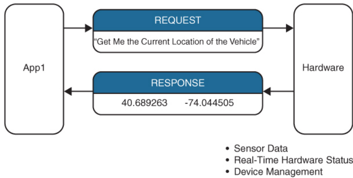
Figure 7-4 Hardware API Providing Access to Hardware in Order to Get or Set Data
