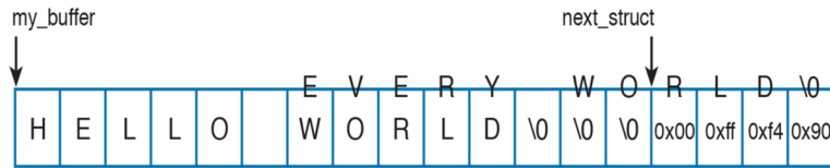
Figure 4-3 A Buffer Overflow
